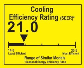
This system's efficiency rating depends on the coil your contractor installs with this unit. The heating efficiency rating varies slightly in different geographic regions. Ask your contractor for details.
